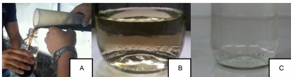
Fig 1. Imagen of the raw material (A), material obtained after a discoloration process (B), material obtained after distillation process (C). The raw material was a crude ethanol obtaining of the fermentation process of the wastewater coffee.
